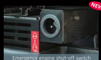
Emergency engine shut-off switch
