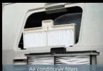
Air conditioner filters
