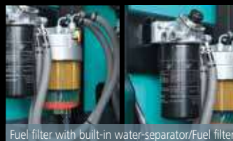
Fuel filter with built-in water-separator/Fuel filter
