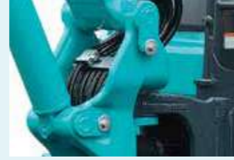
Hydraulic piping The hydraulic piping is housed inside the swing bracket.
