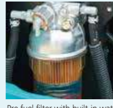
Pre fuel filter with built-in water separator
