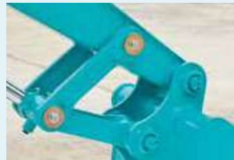
Bucket Cast-iron idler link provide greater strength.
