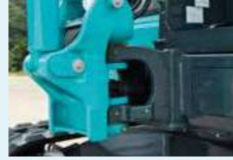
Swing bracket Large, thick cast-iron swing bracket/front bracket.
