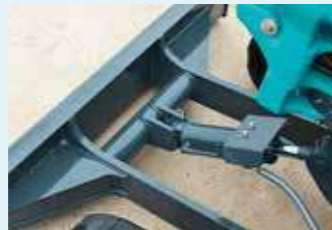
Dozer Box construction dozer supports provide greater strength.
