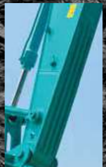
Rock Guards* Specially designed long, solid rock guards installed to prevent damage to arm. *for SK220XD and SK220XDLC
