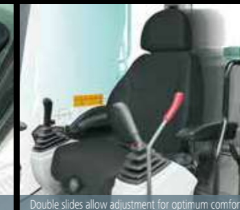
Double slides allow adjustment for optimum comfort
