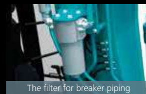
The filter for breaker piping
